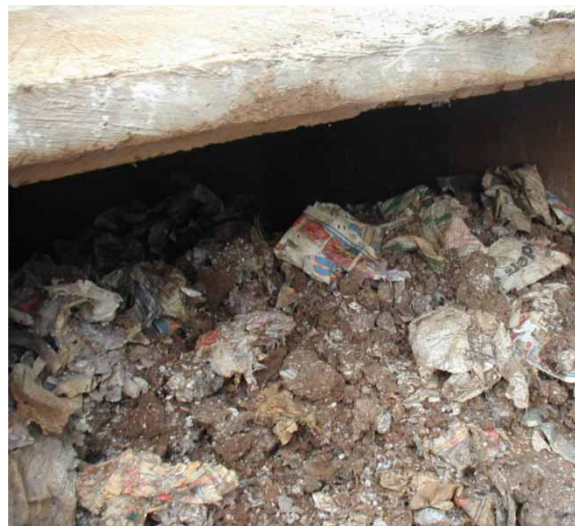
Figure 1 | Variation in physical characteristics and detritus content of faecal sludge, Durban – South Africa.
