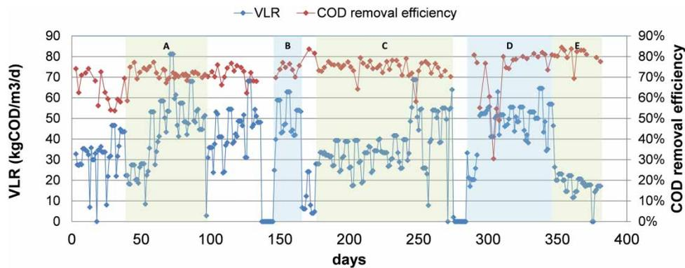
**Figure 3** | Volumetric loading rate and COD removal efficiencies in the ICX demonstration reactor. The periods A-E correspond to those in Table 2.
