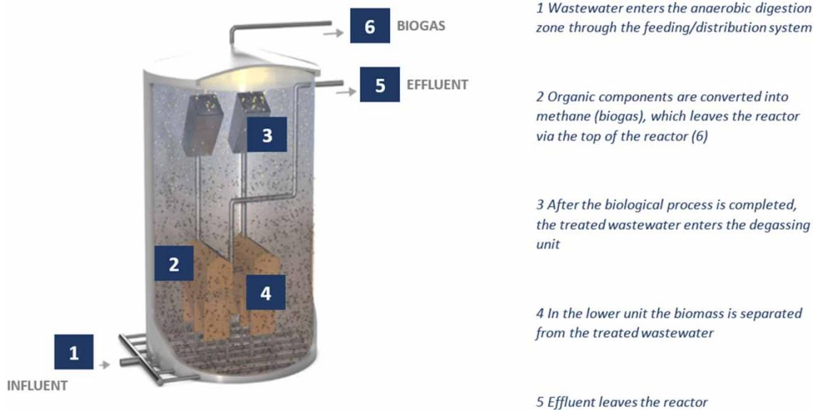
**Figure 1** | Working principle of the Biopaq<sup>®</sup> ICX reactor.
