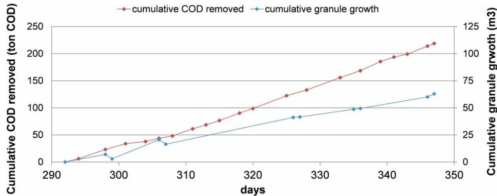
**Figure 4** | Cumulative COD removed and granular biomass growth in the ICX demonstration reactor in period D.
