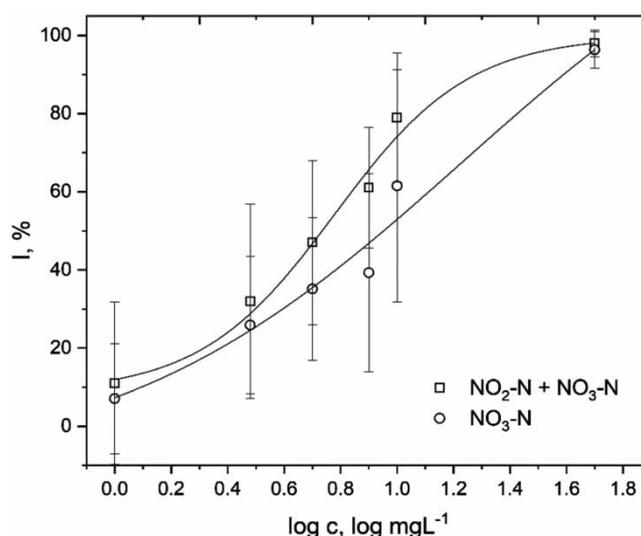
**Figure 2** | Test results of denitrification rate by 3,5-dichlorophenol (3,5-DCP) when inhibition calculations include concentration of  $\text{NO}_3^-$ -N, sum of  $\text{NO}_3^-$ -N and  $\text{NO}_2^-$ -N concentrations. The dark lines show the best dose-response fitting and error bars show the standard deviation of parallel tests ( $n = 7$ ).
