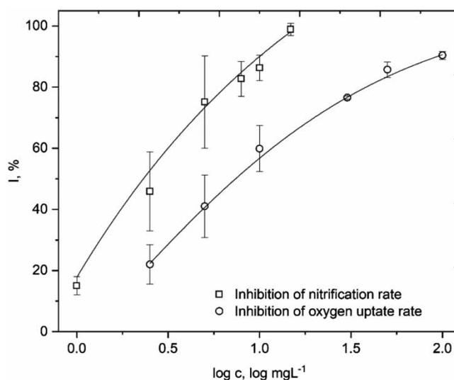
**Figure 1** | Inhibition test results for nitrification rate and total respiration by 3,5-dichlorophenol (3,5-DCP). The dark lines show the best dose-response fitting and error bars show the standard deviation of parallel tests ( $n = 3$ ).
