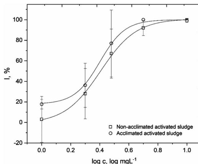
**Figure 3** | Test results of denitrification rate with real industrial wastewater from the oil shale industry with inoculum taken from conventional municipal wastewater treatment plant (MWWTP) and from WWTP where activated sludge is acclimated with phenols and error bars show the standard deviation of parallel tests ( $n = 3$ ).
