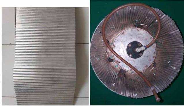
**Figure 6** | Five mm folding width of wall atomizer.
