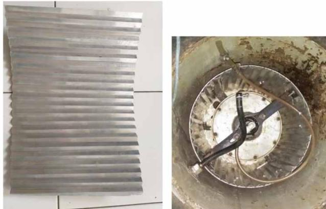
**Figure 8** | Twelve mm folding width of wall atomizer.
