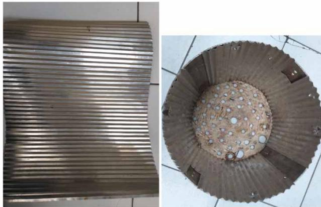
**Figure 7** | Eight mm folding width of wall atomizer.
