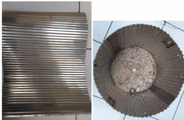
Figure 7 | Eight mm folding width of wall atomizer.
