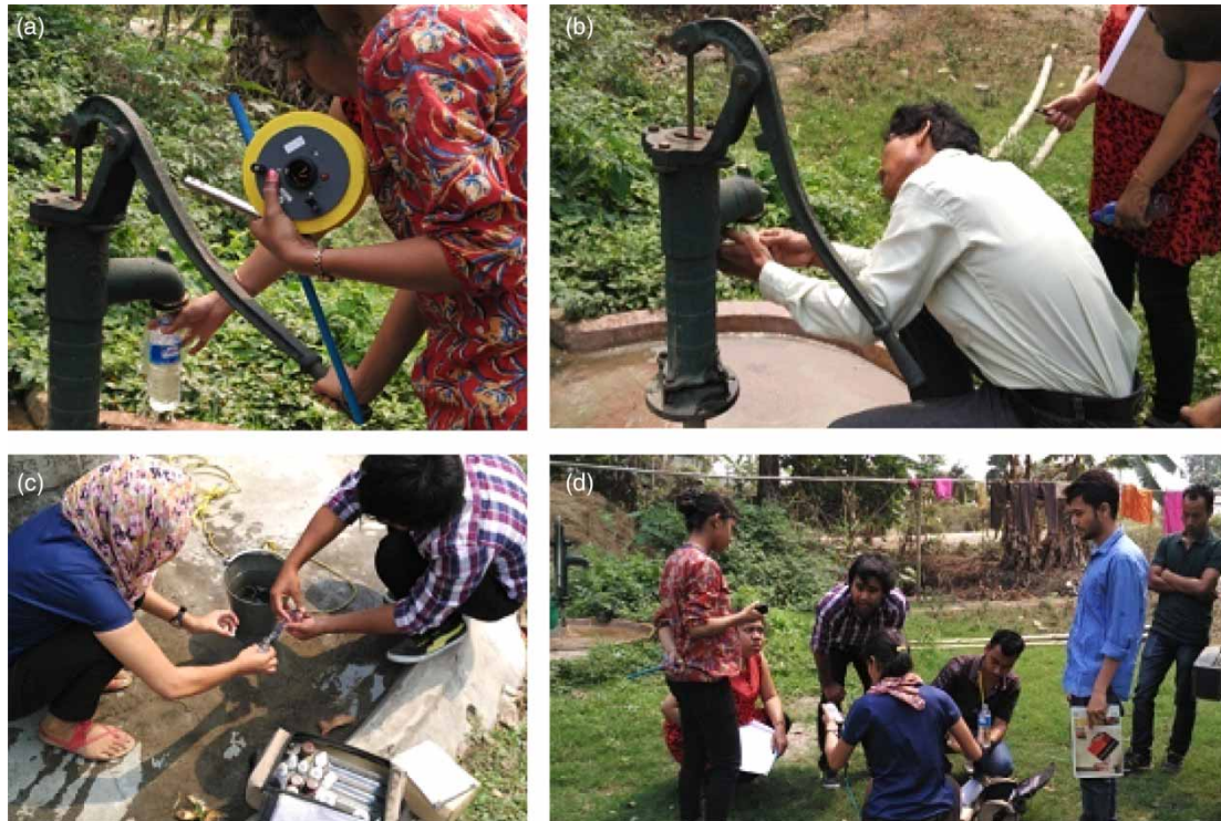
Figure 2 | Sampling campaigns (a) Collecting water samples, (b) Sterilization of hand pump before collecting water sample for bacteriological testing (c) Preparation of groundwater sample (d) Measurement of onsite parameters.
