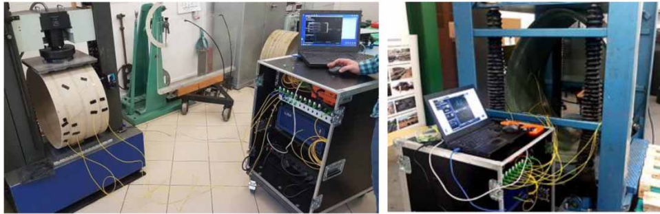
Figure 6 | Test stands for GRP pipe measuring deformation using BOTDR.
