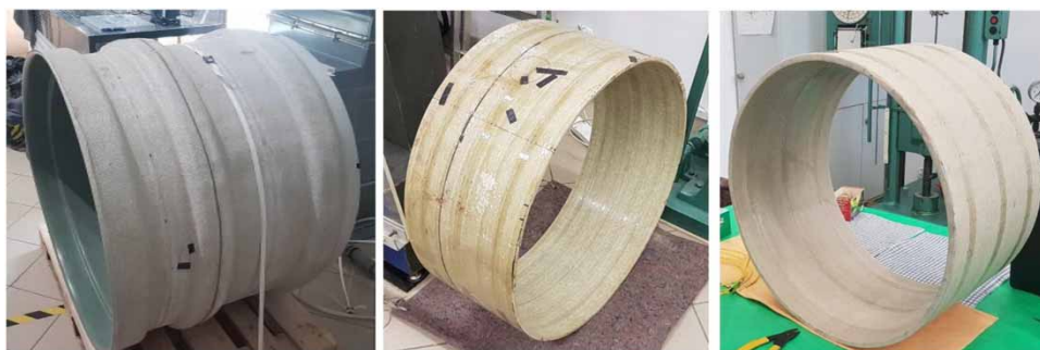
Figure 4 | Pipes with DFOS mounted on outside and inside.
