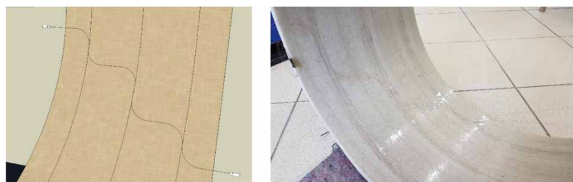
Figure 5 | Fiber optic spacing scheme inside a pipe.
