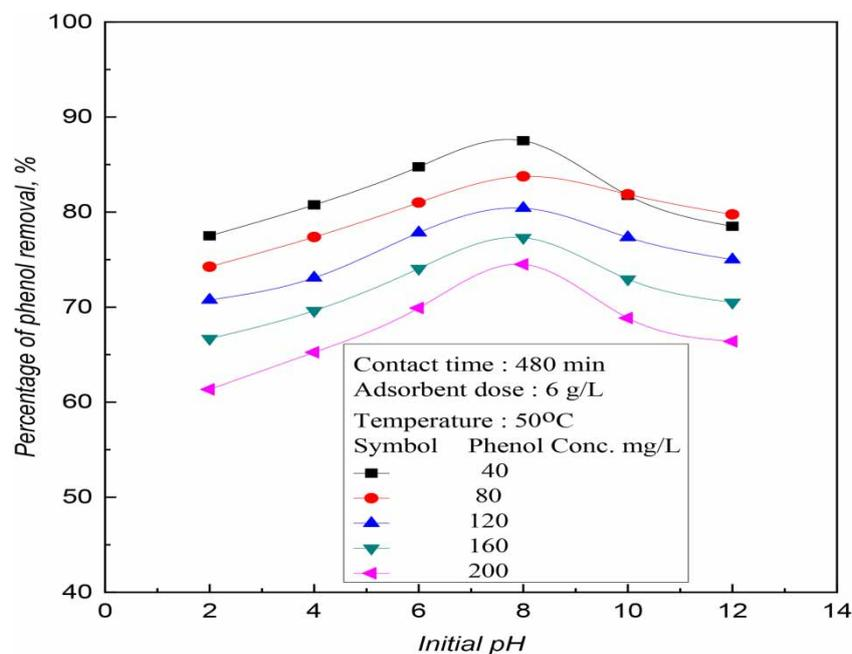
**Figure 6** | The effect of pH for phenol removal.
