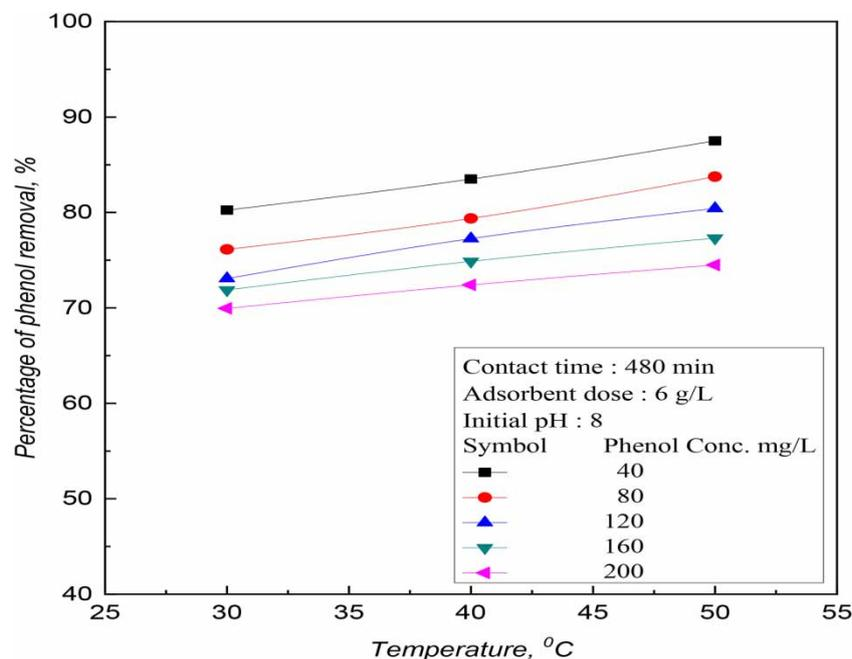
**Figure 7** | The effect of temperature for phenol removal.
