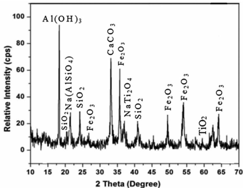
**Figure 2** | The XRD spectra of red mud.
