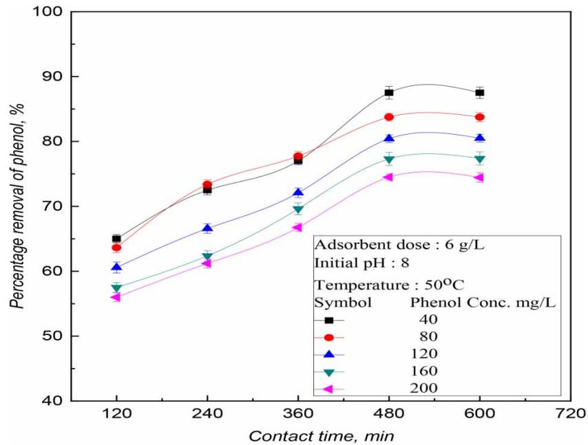
**Figure 4** | The effect of contact time for phenol removal.
