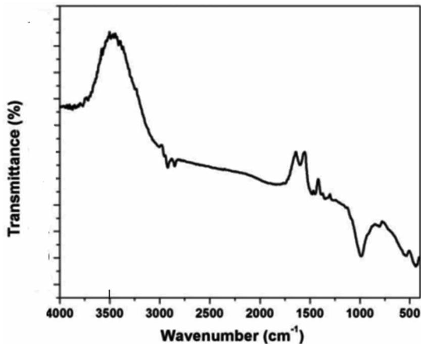
**Figure 3** | The FTIR spectra of red mud.
