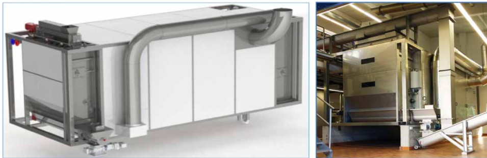
Figure 2 | EloDry ® low temperature dryer – general view and installation at Linz-Unkel.
