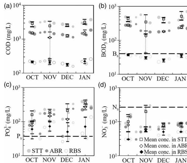
**Figure 2** | Concentration of oxygen demand and nutrients in wastewater at various treatment stages. The size of the bubbles used for STT, ABR and RBS varies because of various HRT. The legends used in panel (c) and (d) are applicable to all panels. The top and bottom whiskers represent the maximum and minimum concentration respectively.  $B_s$ ,  $N_s$  and  $P_s$  refer to the sewage discharge standards for  $BOD_5$ ,  $NO_3^-$  and  $PO_4^{3-}$  respectively in Bangladesh.
