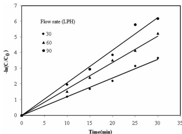
**Figure 3** | Kinetics plot of  $-\ln(C/C_0)$  vs.  $t$  for the batch with recirculation operation of a tubular electrochemical reactor. Current density  $12 \text{ mA/cm}^2$ ; initial concentration  $100 \text{ mg L}^{-1}$ .
