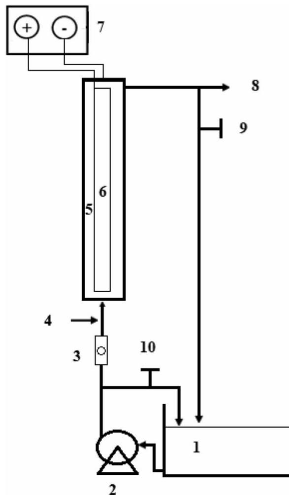
**Figure 2** | Schematic representation of electrochemical reactor. 1 Reservoir, 2 pump, 3 rotameter, 4 tracer injection point, 5 stainless steel cathode, 6 oxide coated mesh type anode, 7 DC power supply, 8 reactor outlet, 9,10 control valve.
