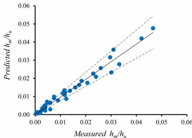
Figure 12 | Comparison between the measured  $h_m/h_u$  and that predicted by Equation (7), and  $\pm 20\%$  prediction range.
