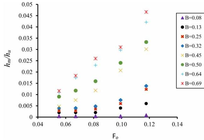
Figure 11 |  $h_m/h_u$  versus  $F_o$  for various blockage ratios.
