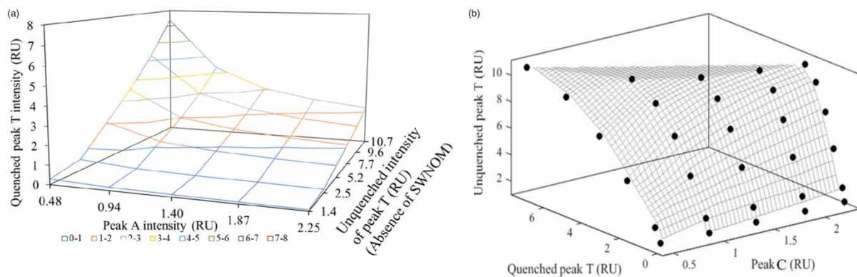
**Figure 3** | (a) Effect of BSA and SWNOM concentration on peak T's quenched intensity. BSA concentration presented in terms of peak T's unquenched intensity, T (RU); SWNOM concentration in terms of peak C (RU). (b) Relationship between BSA's unquenched peak T and its quenched peak T and peak C (the grid pane is for visualization of the data pattern).
