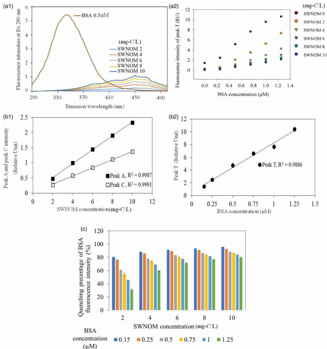
**Figure 2** | (a1) Overlapping fluorescence spectrum of SWNOM and BSA, (a2) fluorescence peak intensity of BSA in the presence of varying concentrations of SWNOM; (b) relationship between fluorescence peak intensity and varying concentrations of (b1) SWNOM, and (b2) BSA. (c) Quenching percentage of BSA fluorescence intensity at different concentrations of BSA and SWNOM.
