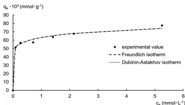
Figure 8 | MB adsorption isotherms on RH-1.
