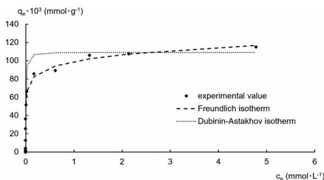
Figure 9 | MB adsorption isotherms on RH-2.
