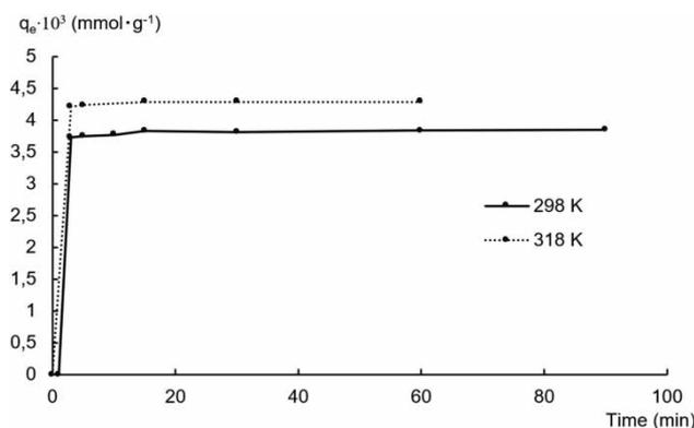
**Figure 6** | Effects of contact time on RH-2 MB removal efficiency at different temperatures.
