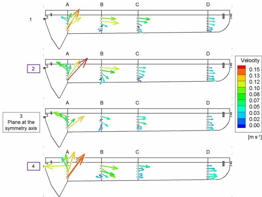
**Figure 4** | Velocity distribution of the vectors  $u-w$  in the four longitudinal sections at  $q_{A2} = 9.5 \text{ m h}^{-1}$  (the cross-sections 2 and 4 (marked by purple frames) may be compared as ones on opposite sides of the symmetry axis). The full colour version of this figure is available in the online version of this paper, at <http://dx.doi.org/10.2166/wpt.2021.006>.
