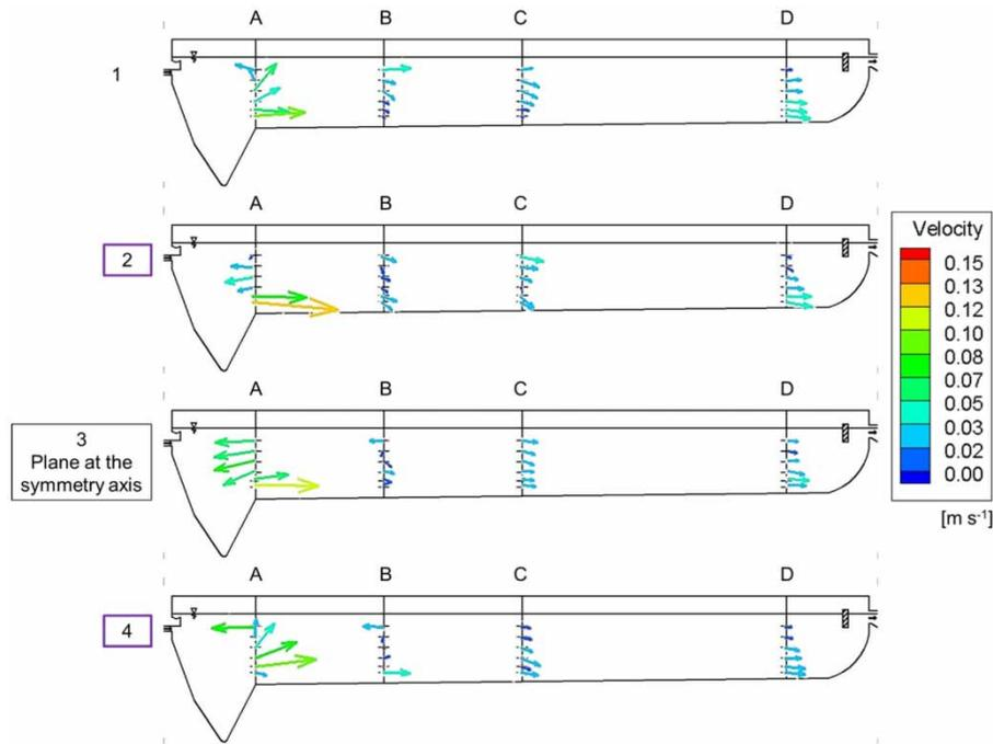
**Figure 2** | Velocity distribution of the vectors of  $u-w$  in the four longitudinal sections at  $q_{A1} = 5 \text{ m h}^{-1}$ . The cross-sections 2 and 4 (marked by purple frames) may be compared to the ones on opposite sides of the symmetry axis. The full colour version of this figure is available in the online version of this paper, at <http://dx.doi.org/10.2166/wpt.2021.006>.
