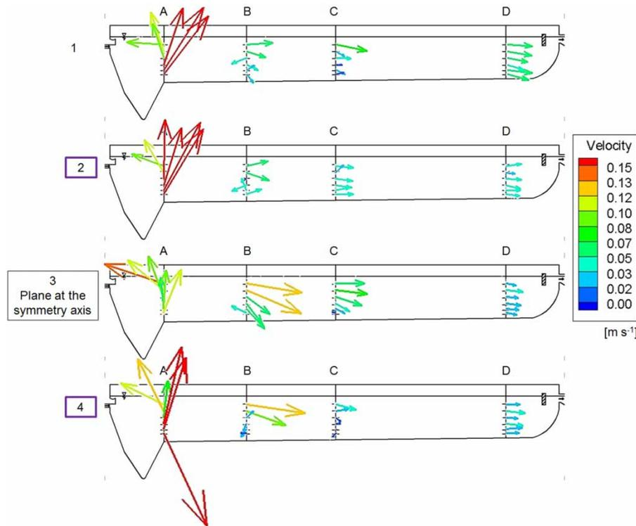
**Figure 6** | Velocity distribution of the vectors of  $u-w$  in the four longitudinal sections at  $q_{A3} = 13 \text{ m h}^{-1}$  (the cross-sections 2 and 4 (marked by purple frames) may be compared as ones on opposite sides of the symmetry axis). The full colour version of this figure is available in the online version of this paper, at <http://dx.doi.org/10.2166/wpt.2021.006>.
