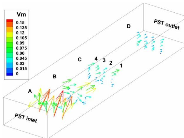
**Figure 5** | 3D images of resultant velocity vectors [ $\text{m s}^{-1}$ ] at  $q_{A2} = 9.5 \text{ m h}^{-1}$ .
