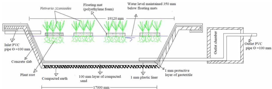
**Figure 2** | FCW cross-section.
