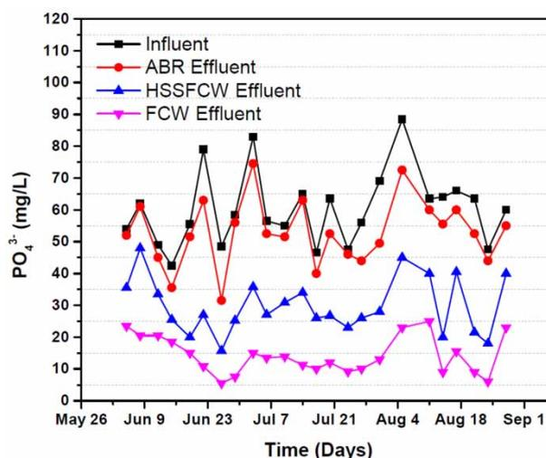
**Figure 5** | Variation in phosphate concentration by stage through time.
