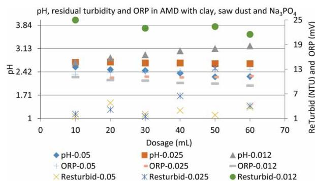
**Figure 3** | pH, residual turbid materials and ORP of treated AMD sample dosed with varying concentration of Na<sub>3</sub>PO<sub>4</sub> in the flocculant.
