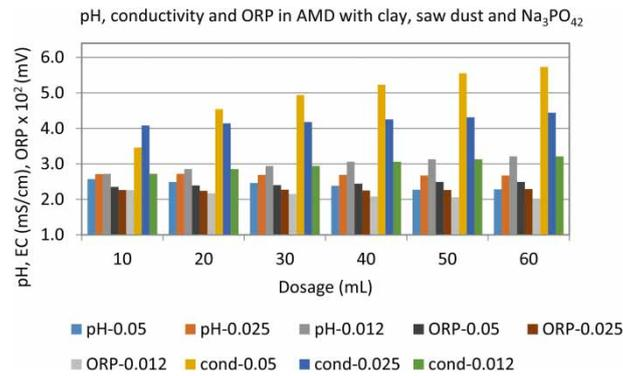
**Figure 2** | pH, conductivity and ORP of AMD sample with varying dosage of clay, saw dust and Na<sub>3</sub>PO<sub>4</sub>.
