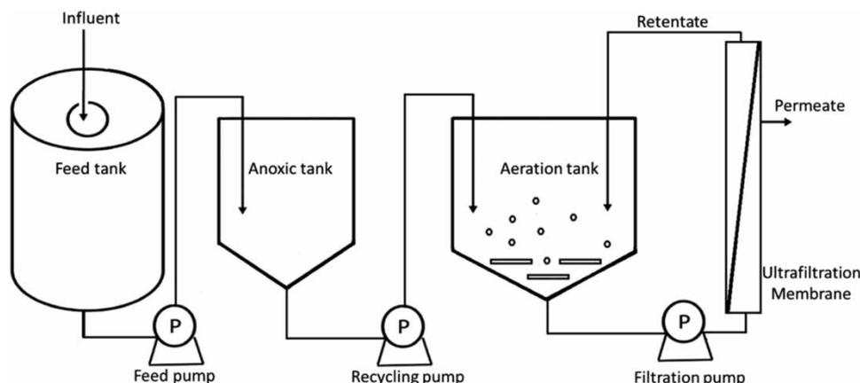
Figure 1 | Schematic diagram of ultrafiltration module.
