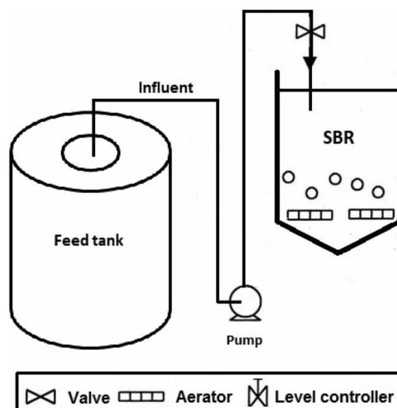
**Figure 2** | Schematic diagram of SBR pilot.
