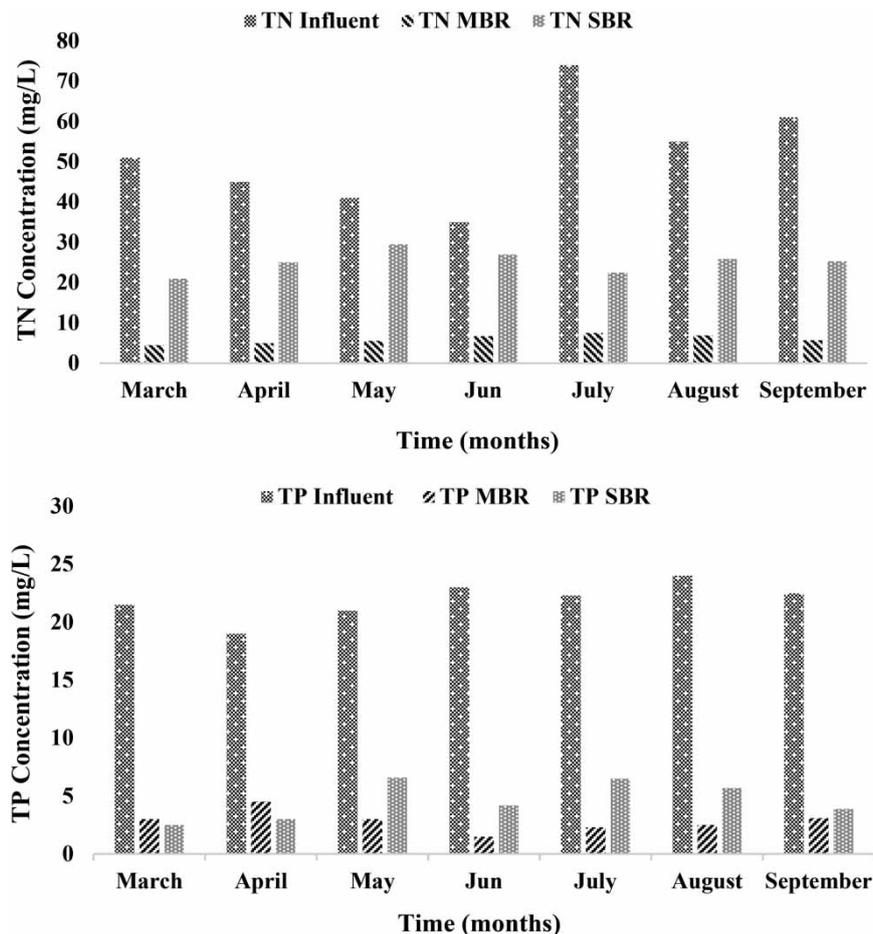
**Figure 5** | TN and TP concentrations average value in the influent, MBR and SBR effluent.
