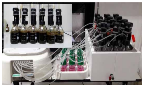
Figure 1 | Automatic anaerobic digestion methane potential test system.
