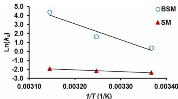
**Figure 9** | Plot of  $\ln K_d$  vs.  $1/T$  for NZP adsorption on SM and BSM adsorbents.
