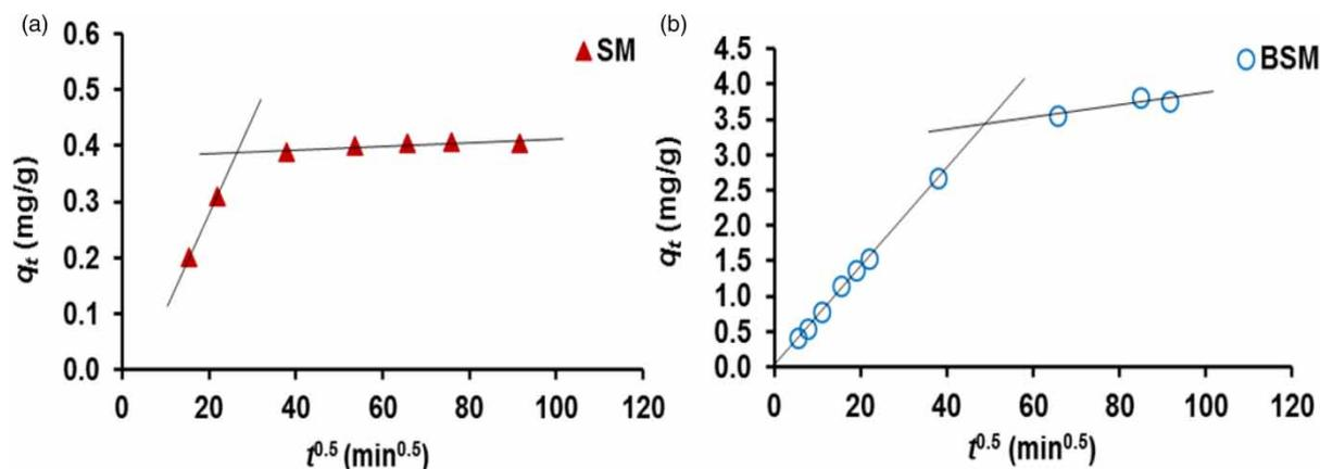
**Figure 8** | Intra-particle diffusion plots for NZP adsorption on (a) SM and (b) BSM adsorbents at 24 °C.
