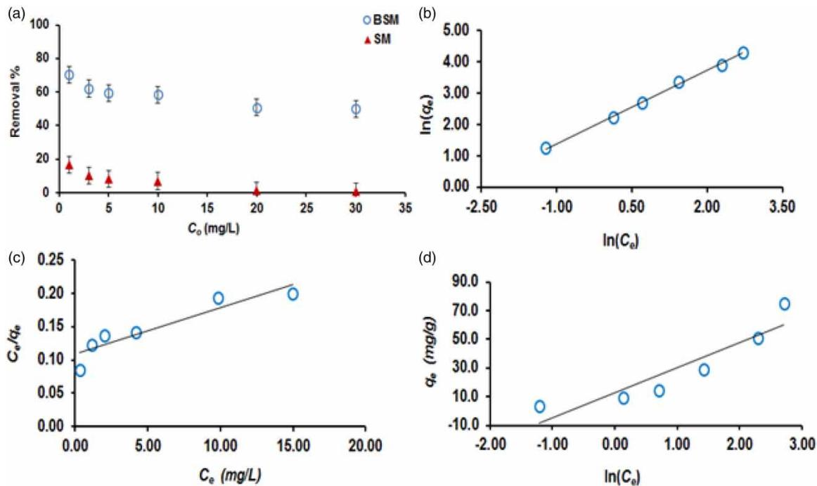
**Figure 5** | (a) effect of NZP concentration on the removal efficiencies of SM and BSM adsorbents at a 24 °C, linear least squares fit of (b) Freundlich model, (c) Langmuir model and (d) Temkin model.
