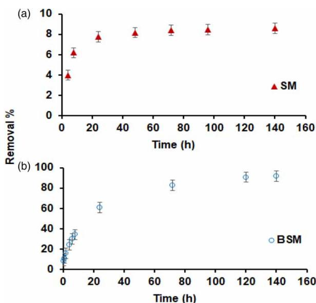
**Figure 6** | Contact time effect on the removal efficiency of (a) SM and (b) BSM for NZP. Concentration of NZP is 5 mg/L, adsorbent dosage concentration is 1 g/L and shaking speed is 140 rpm at a temperature of 24 °C.
