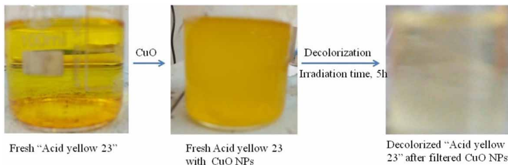
Figure 4 | Shows the decolorization test, for the acid yellow 23 as model dye, using 20 mg CuO NPs in the presence of visible light for the irradiation time of 5 h was performed in the laboratory.
