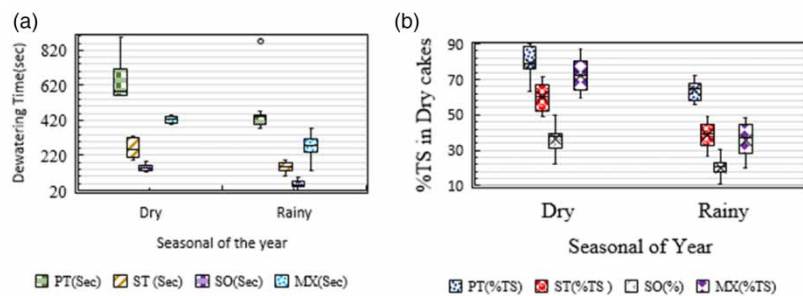
Figure 4 | Box plots illustrating the seasonal variability of dewatering time performance (CST (SL/GTS)) and dewatering extent (%TS in dry cakes) performance in different containments. (a) Dewatering rate performance for FS dewatering, (b) dewatering extent performance for FS dewatering.
