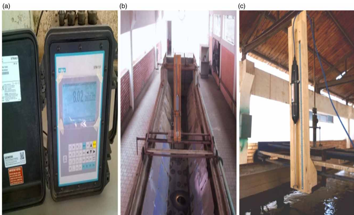
Figure 3 | The experimental tools. (a) Current flow meter/ uniflow universal; portable flow meter. (b) Measuring levels: point gauge. (c) Vectrino 3D water velocity sensor.
