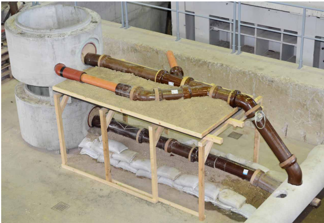
Figure 3 | Connection lines with the lower line to be inspected with four damage patterns.
