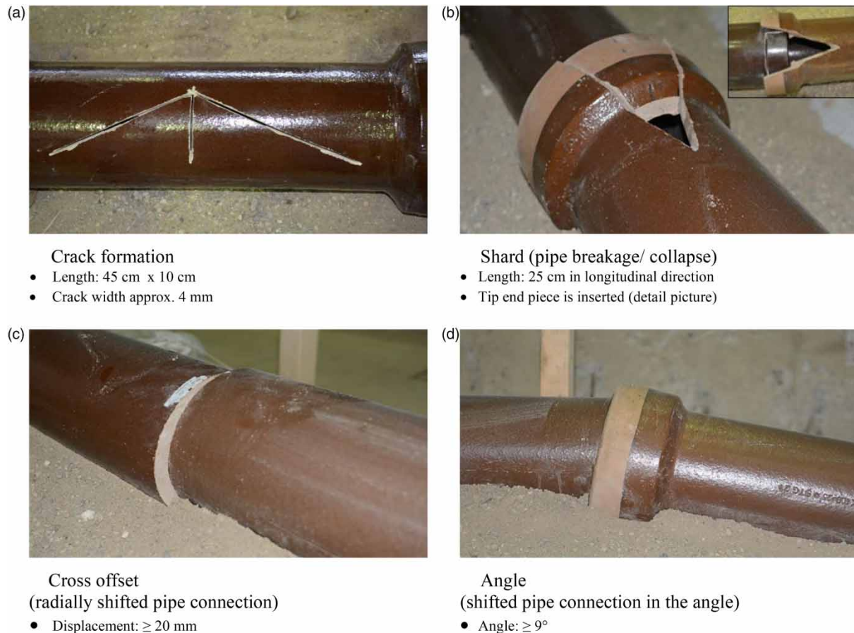
Figure 4 | Built-in large damages (a-d) for performing the visual inspection (Bosseler et al. 2018).
