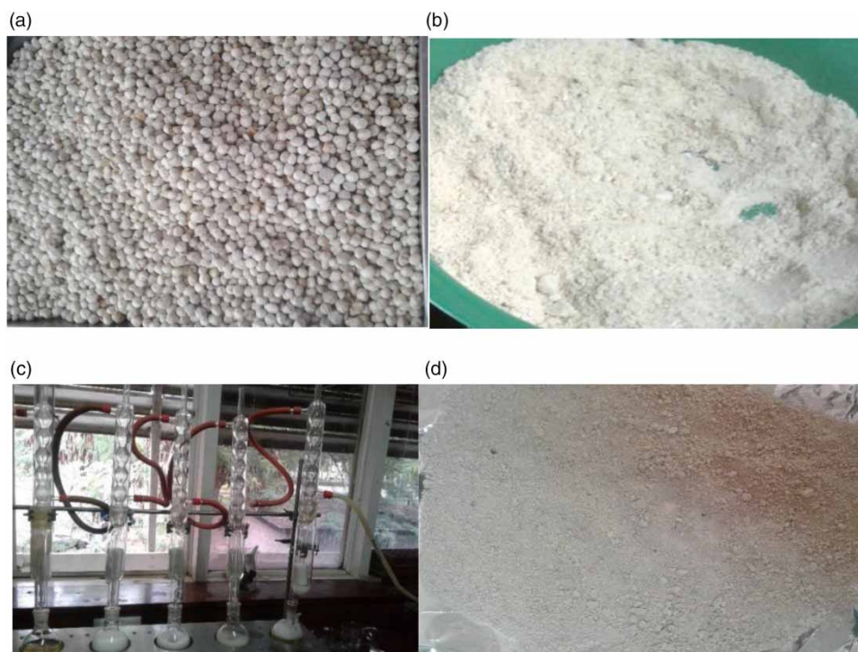
Figure 2 | Preparation of Moringa Oleifera seeds powder. (a) Deshelled MO seeds, (b) MO seeds powder, (c) oil extraction from MO seeds powder, and (d) yield of MO seeds powder.
