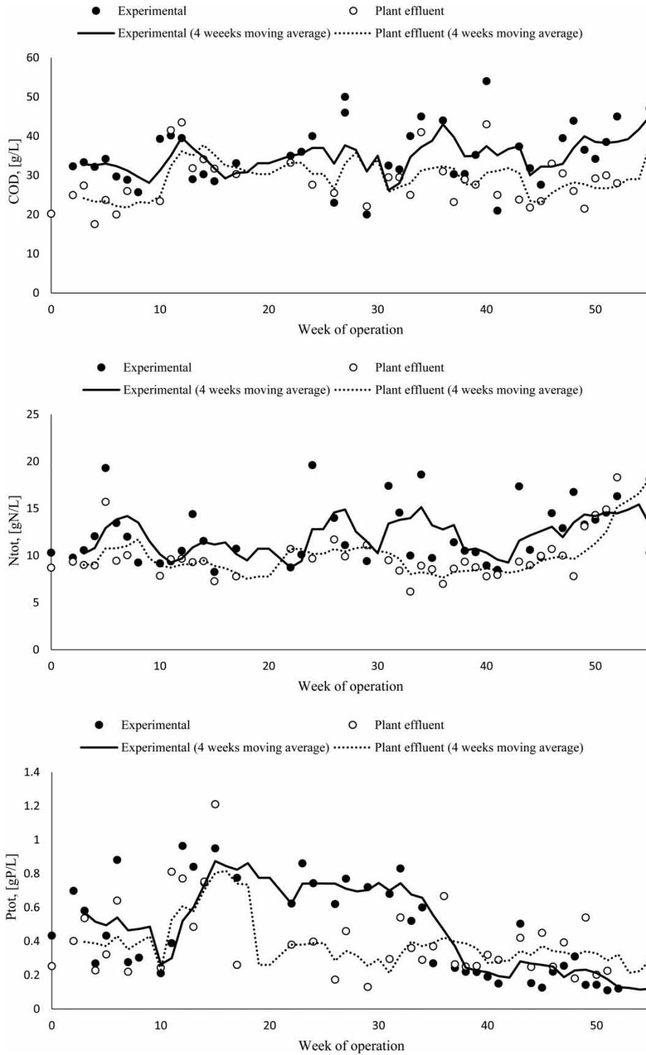
**Figure 2** | Effluent quality (COD, N<sub>tot</sub>, P<sub>tot</sub>) in experimental process train compared to plant effluent.
