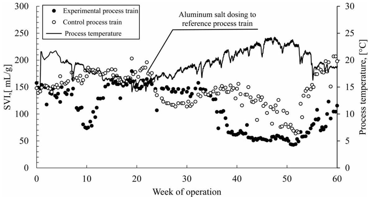
**Figure 3** | SVI<sub>30</sub> variations in experimental and reference process train.
