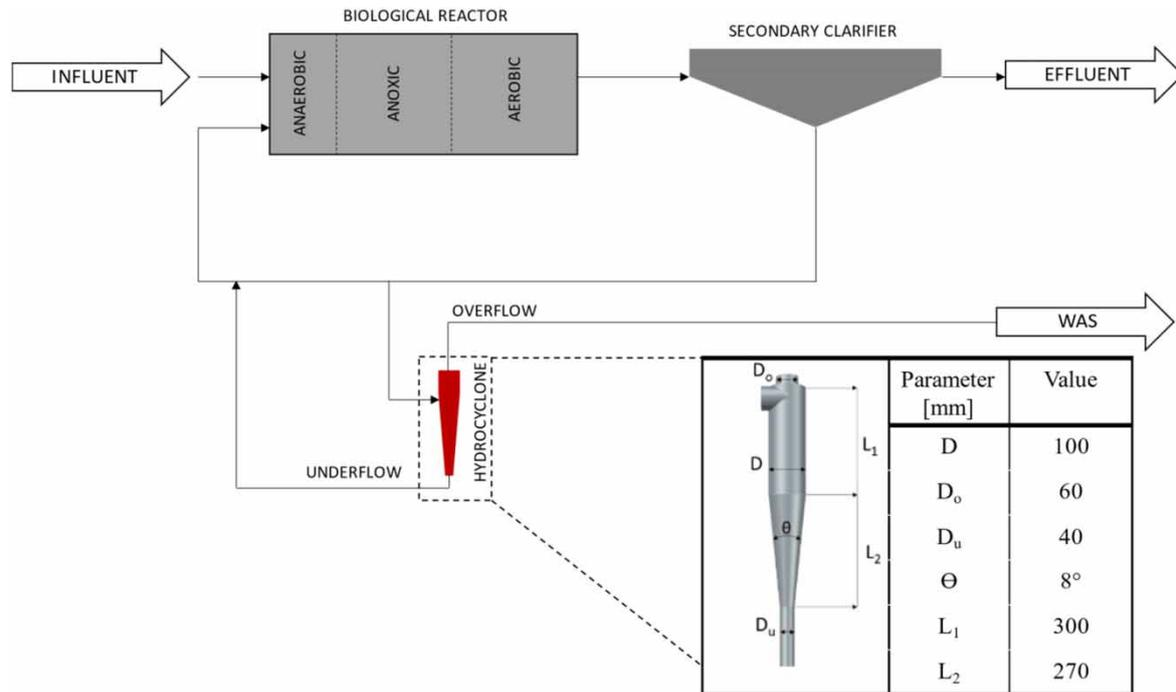
**Figure 1** | Flow diagram of activated sludge process with gravimetric selection technology.
