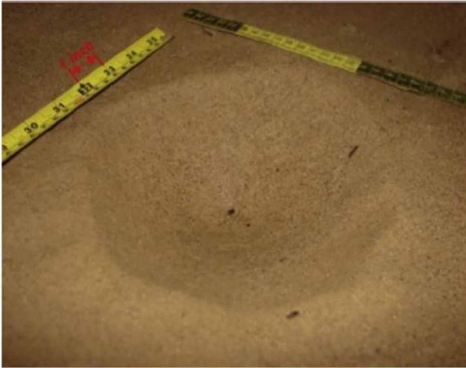
Figure 5 | Scour hole formed in fine sediment for C = 2.5 cm. (Asiaban et al. 2017).
