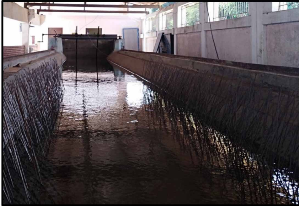
Figure 1 | Artificial canal, with rigid vegetation on the channel side slopes.
