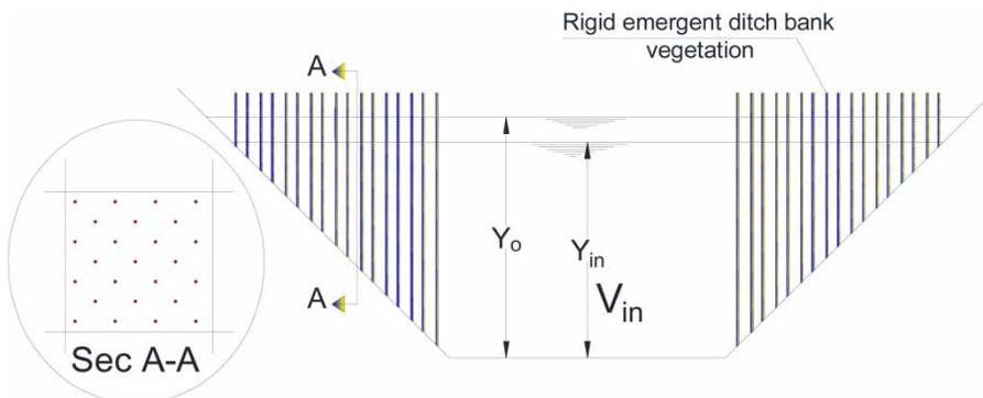
**Figure 4** | Cross-section of the vegetated reach.
