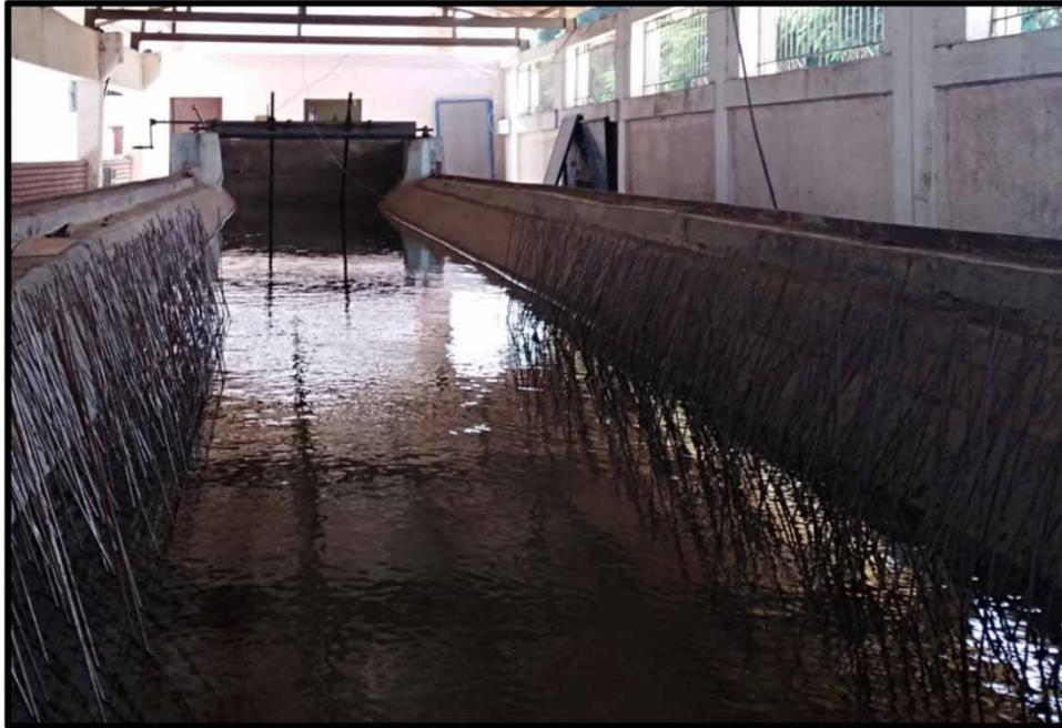
**Figure 1** | Artificial canal, with rigid vegetation on the channel side slopes.
