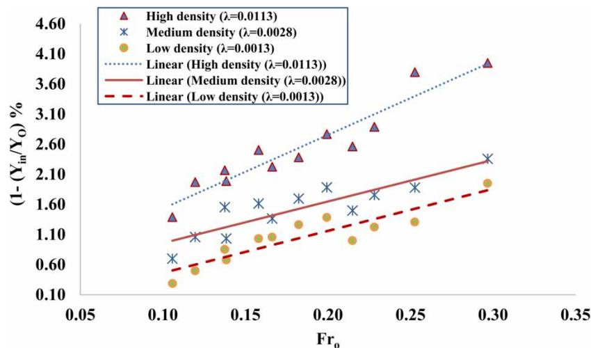
**Figure 6** | Relationship between water depth reduction ( $Y_{in}/Y_o$ ) within the vegetated reach and  $Fr_0$  in the unvegetated case.
