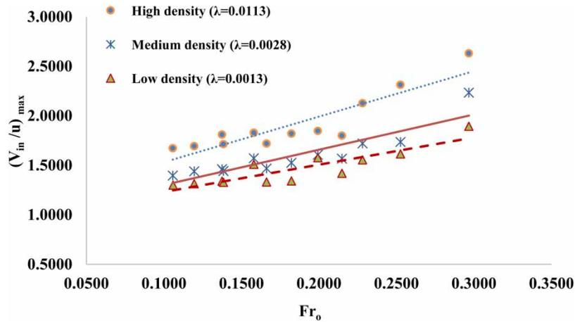
**Figure 10** | Relationship between  $V_{in}/u_{max}$  and  $Fr_o$  in the unvegetated case.
