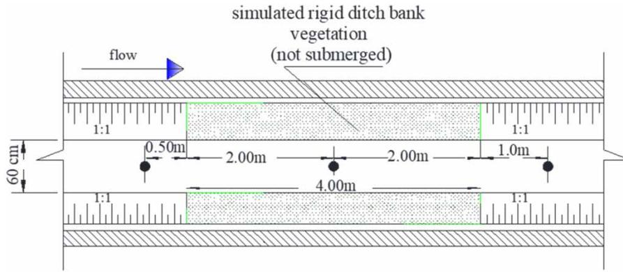
**Figure 3** | Velocity measuring points upstream, within, and downstream of the vegetated reach.
