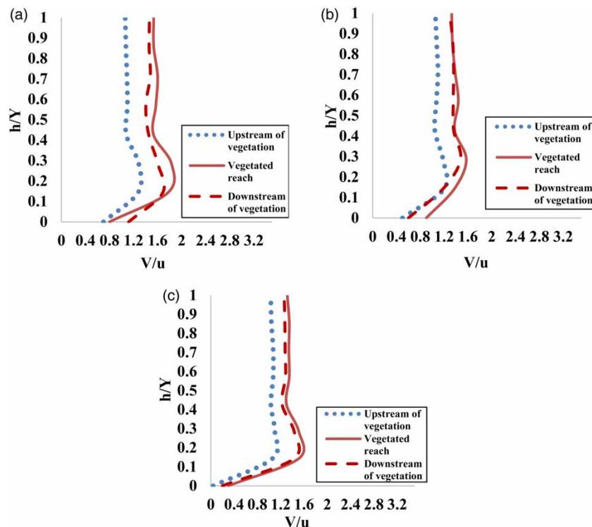
**Figure 7** | Velocity profiles for different vegetation densities ( $\lambda$ ) at  $Q=40$  l/s and  $Fr_o=0.15$ , for (a)  $\lambda=0.0113$ , (b)  $\lambda=0.0028$ , and (c) For low  $\lambda=0.0013$ .
