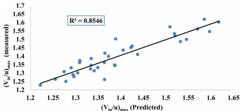
**Figure 12** | Comparison between measured and predicted  $(V_{in}/u)_{max}$
