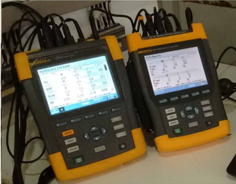
Figure 14 | Fluke® energy analyzer.
