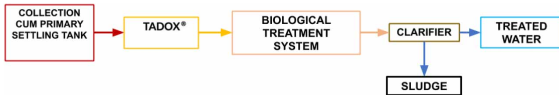
Figure 1 | Schematic showing TADOX ® Implementation at Pre-Biological Stage.
