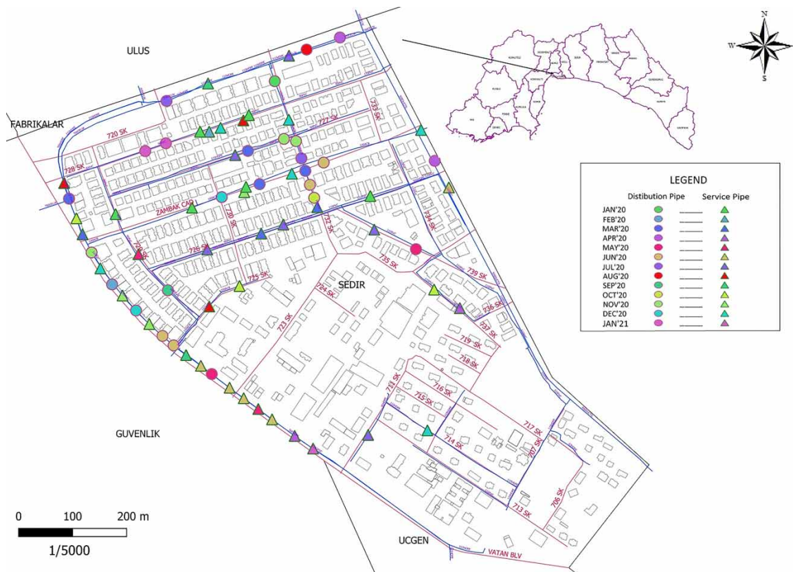
Figure 4 | Locations and types of pipe failures in the PSA.
