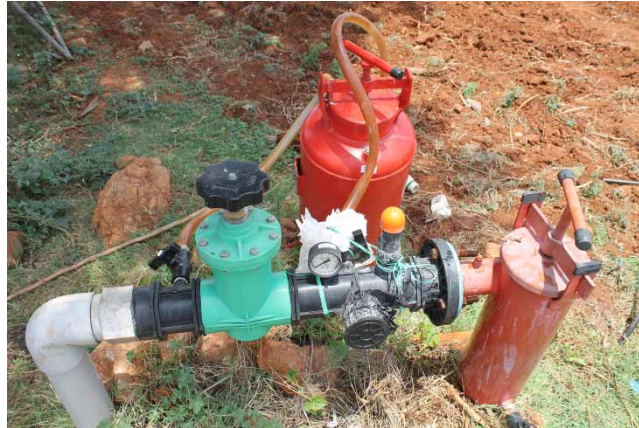
Figure 2 | Fertigation equipment connected to the drip irrigation system (representative picture).
