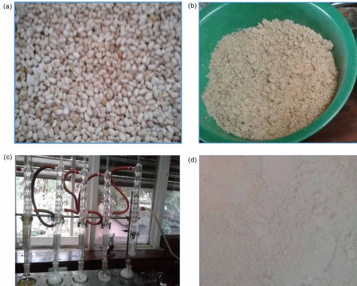
Figure 5 | Preparation of JC seed powder. (a) JC seeds; (b) oil JC powder; (c) the Soxhlet method for oil extraction; and (d) 0.58-mm sieved fine particles.
