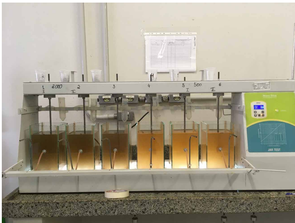
Figure 2 | Jar test equipment with ash dispersion in three flasks.
