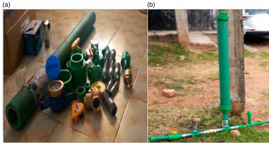
Figure 5 | Fabrication of the hydram pump: (a) components and (b) complete hydram pump.
