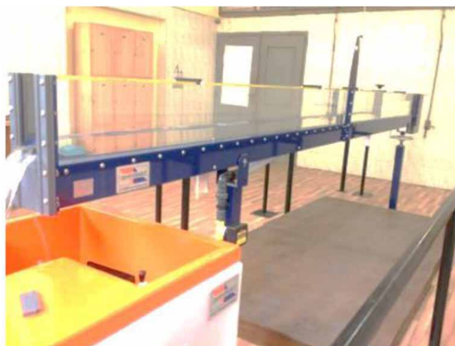
Figure 1 | The flume and the hydraulic bench.
