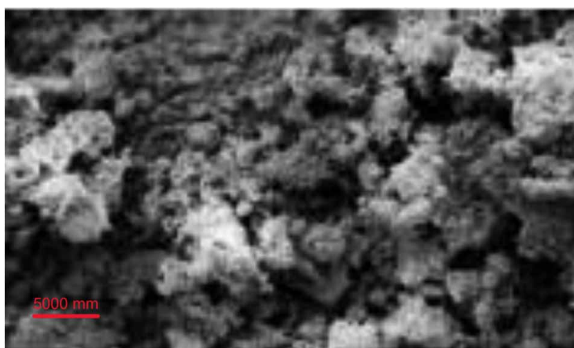
Figure 12 | SEM image of AC950-240, magnification 5,000 ×.
