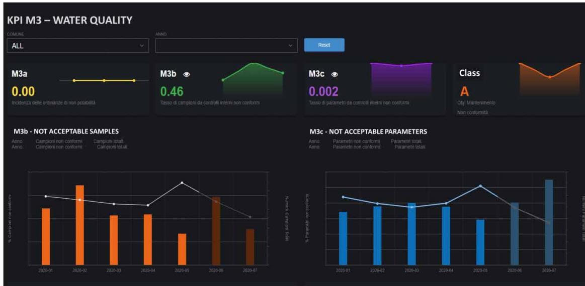
Figure 4 | The dashboard shows water quality KPIs in water networks related to sampling activity and laboratory analysis. Based on the number of not acceptable water samples and water quality parameters, it calculates the class for each municipality (from A to E with A being the best).
