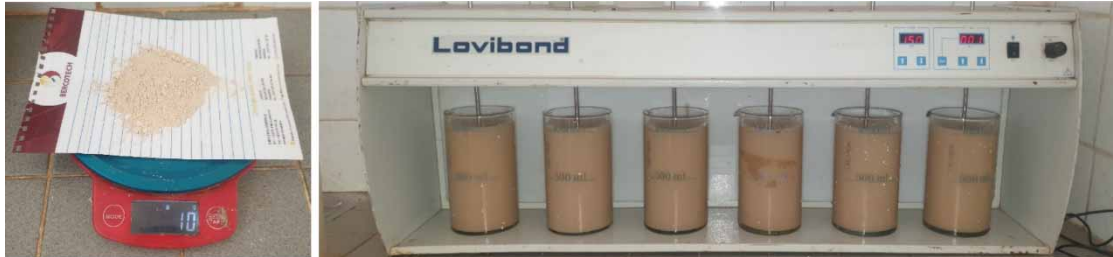
Figure 2 | Preparation of synthetic turbid water.
