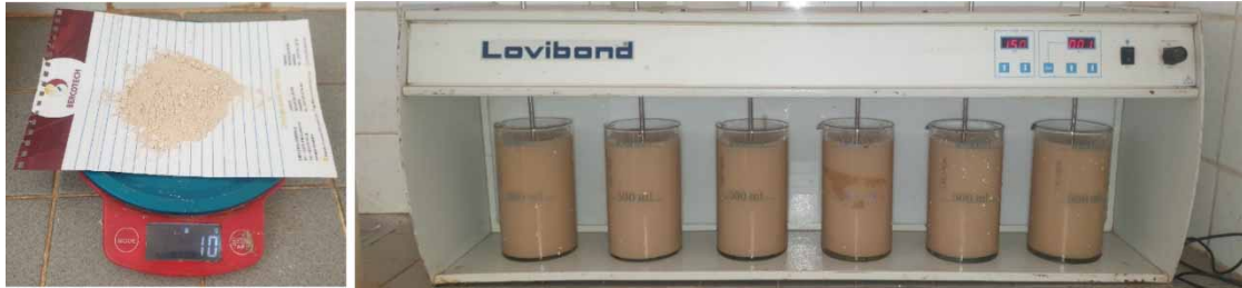
Figure 2 | Preparation of synthetic turbid water.
