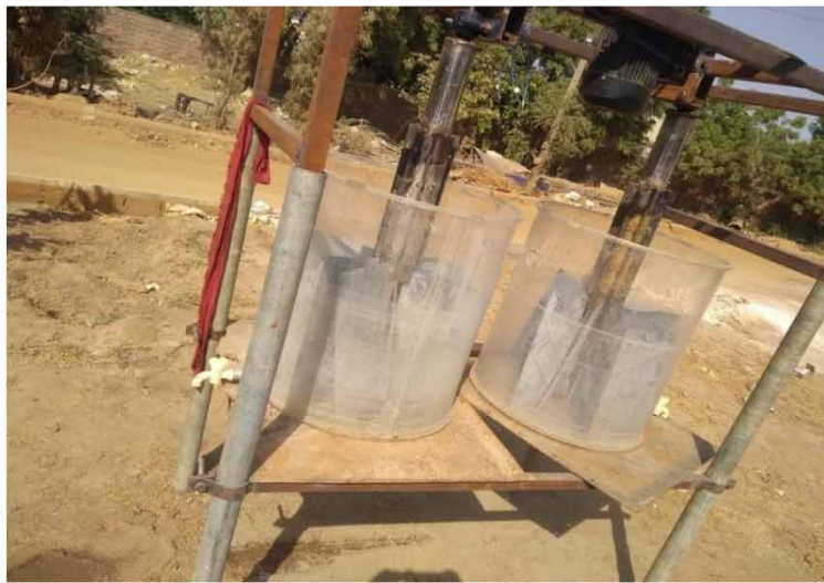
Figure 2 | ZnO-based fabricated photocatalytic reactor: (a) schematic diagram and (b) field setup.
