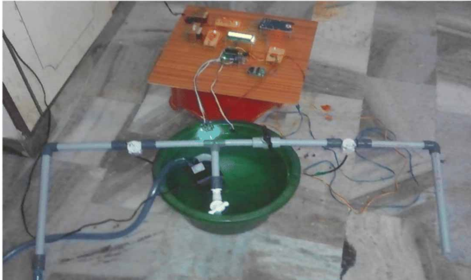
Figure 10 | Experimental results of water flow detection – no leak.
