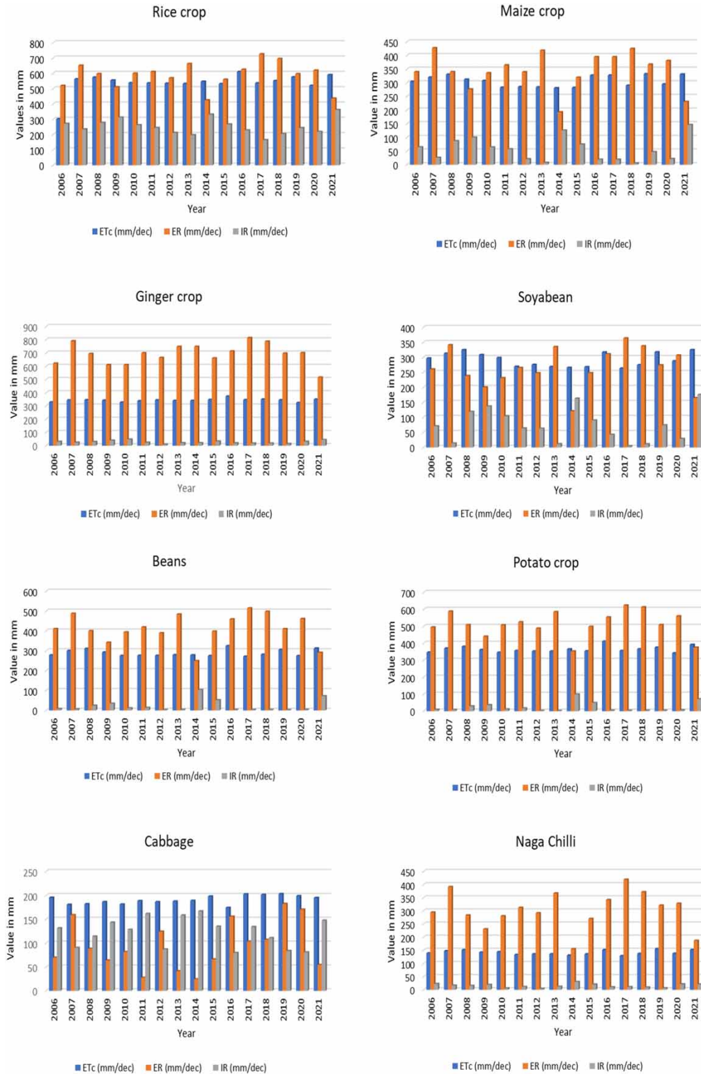
Figure 3 | ET c , effective rainfall, and irrigation requirements of different crops grown at Kohima.
