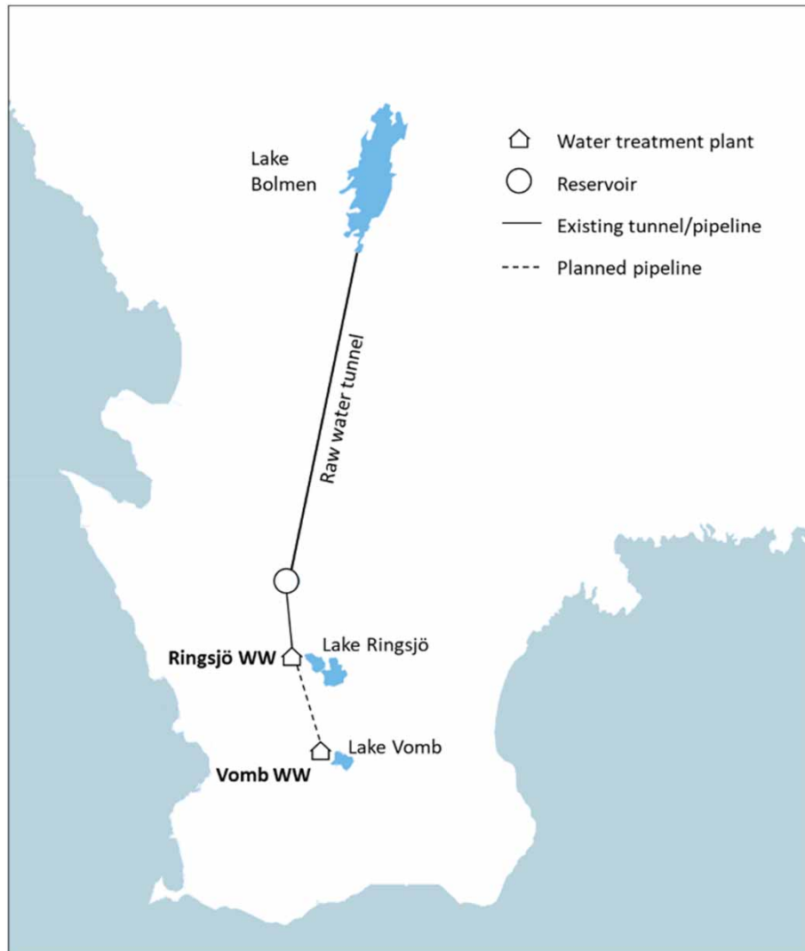
Figure 1 | Overview of Southern Sweden Water Supply's source, WWs and planned raw water pipeline. The figure shows the three raw water sources – Lake Bolmen, Lake Ringsjö and Lake Vomb – and the two main WW – Ringsjö and Vomb (adapted from Sydvatten (2018) ).
