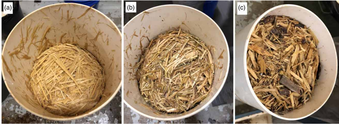
Figure 3 | Lab-scale bioreactors filled with (a) barley straw (b) hemp straw and (c) woodchips (view from top, 15 cm in diameter).
