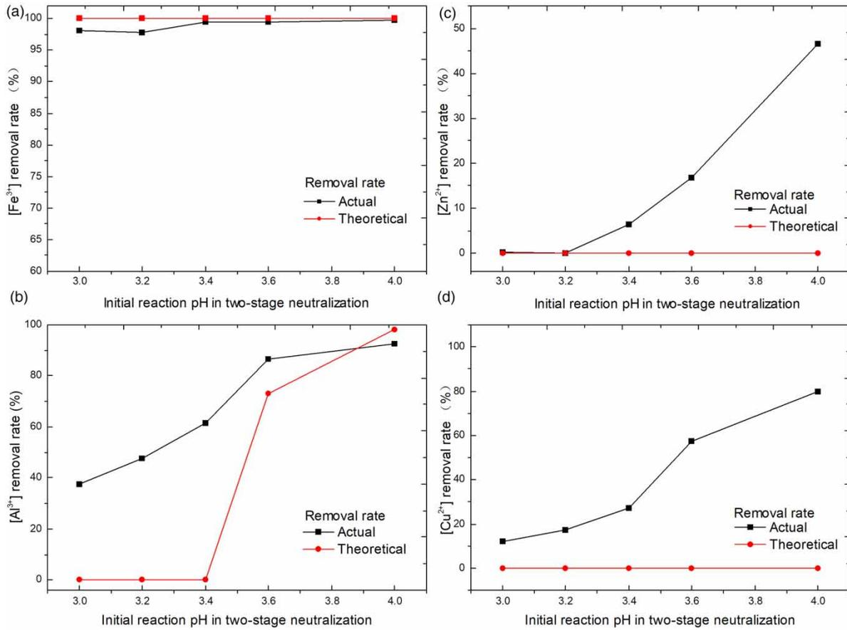
**Figure 5** | Effect of pH on actual and theoretical removal rates of Fe<sup>3+</sup> (a), Al<sup>3+</sup> (b), Zn<sup>2+</sup> (c) and Cu<sup>2+</sup> (d).
