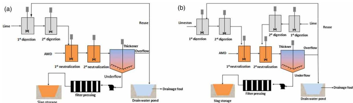
**Figure 2** | Neutralization flowcharts – (a) single-stage (b) two-stage.
