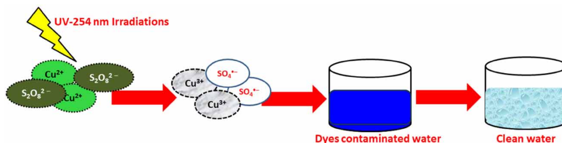
Figure 9 | Proposed mechanism of activation of the UV/Cu 2+ /PDS system for degradation of MO and MV dyes.
