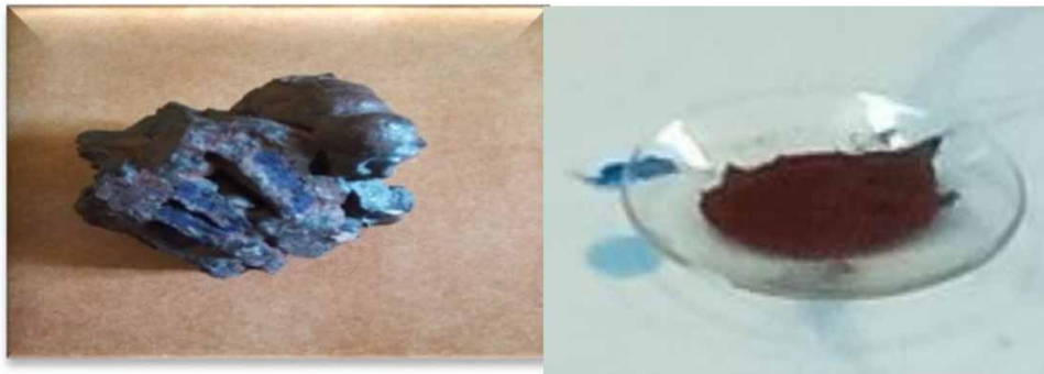
Figure 1 | Tested goethite (laboratory photo).
