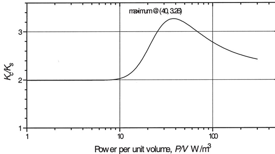
**Fig. 5.** Relative performance of circular and square tank aerators on oxygen transfer coefficient,  $k$ , for any given input power per unit volume.
