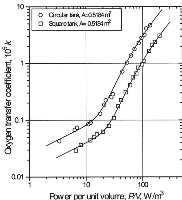
Fig. 4. Power requirements to aerate same volume of water in circular and square tank aerators.
