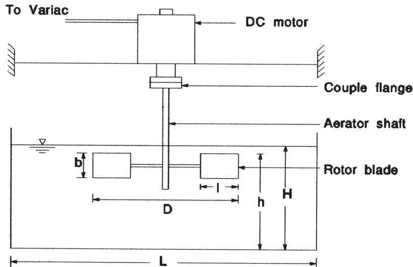
Fig. 1. Schematic diagram of aerator.
