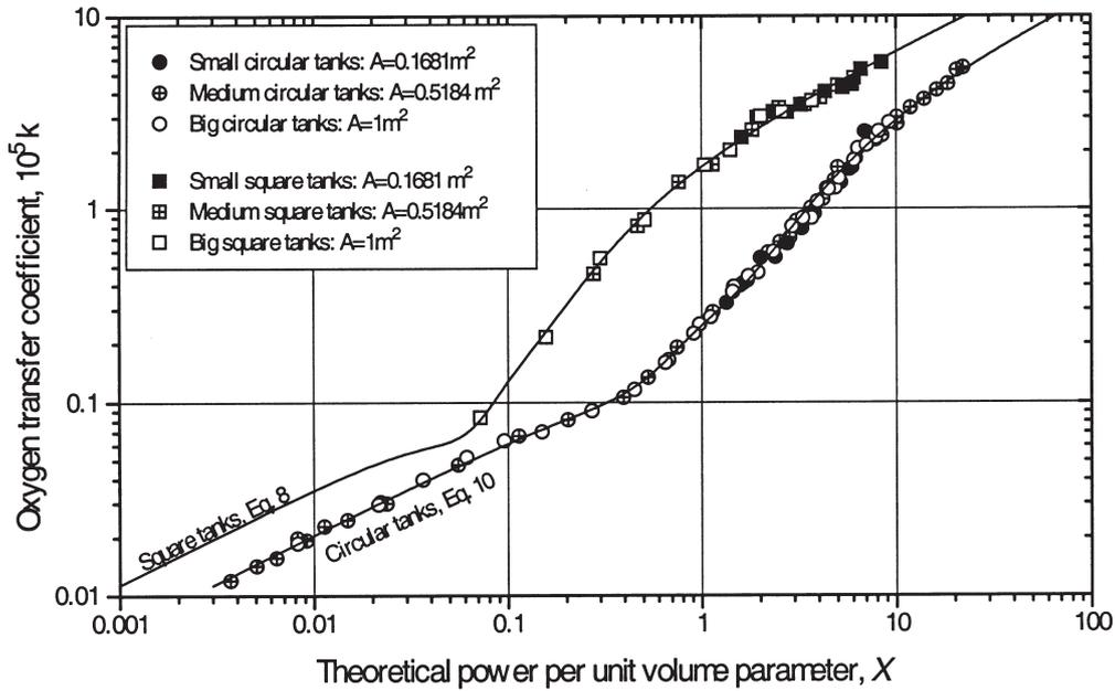
Fig. 2. Simulation of oxygen transfer in circular tanks along with square tanks.
