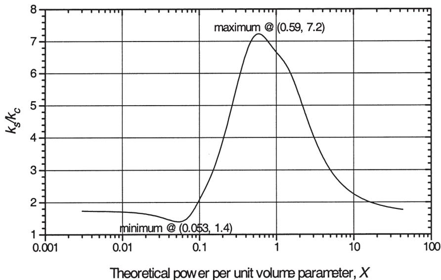
Fig. 3. Relative performance of circular and square tank aerators on oxygen transfer parameter,  $k$ , for any given  $X$ .
